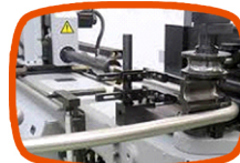
Semi Automatic Pipe Bending
